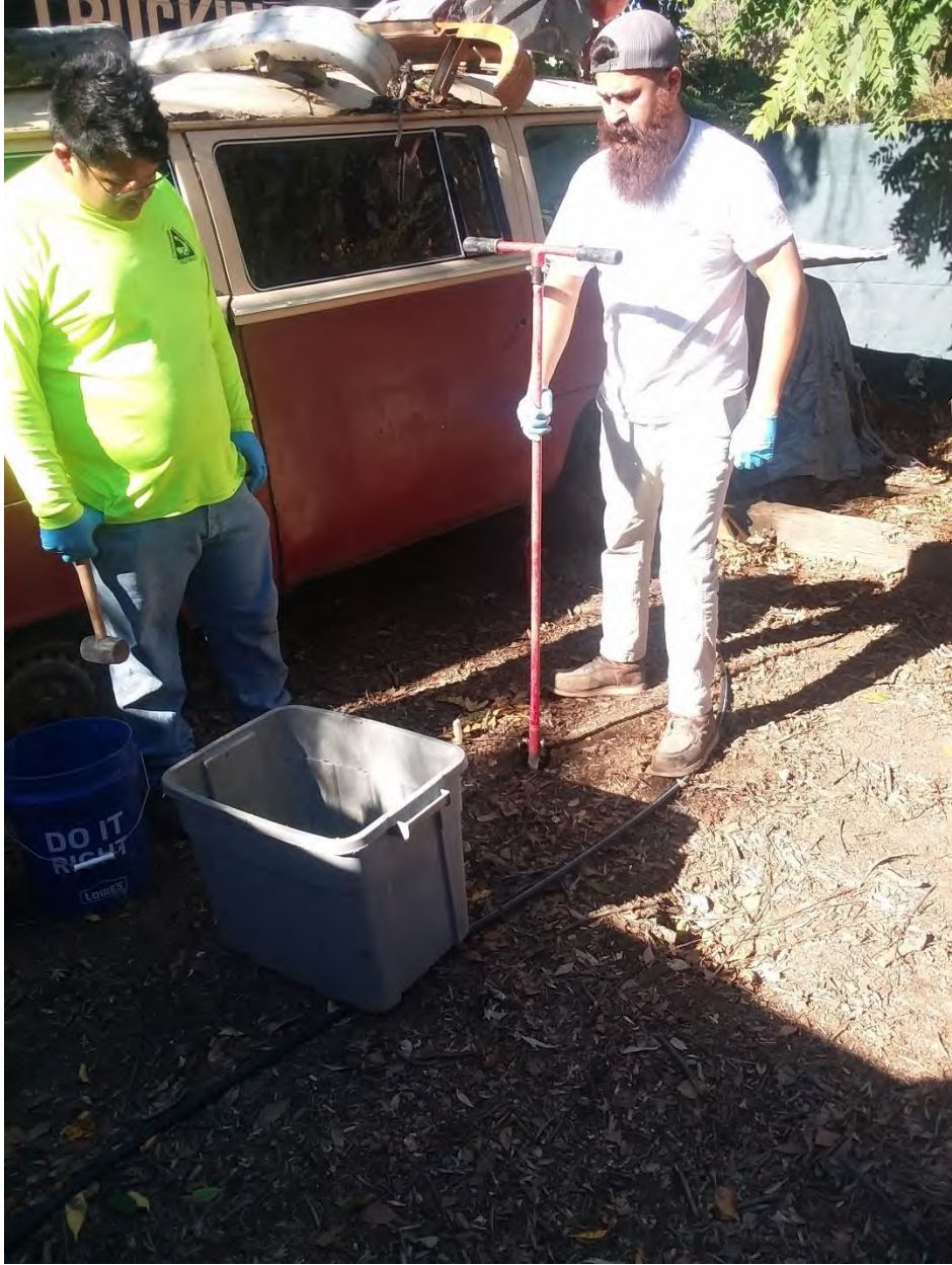
Photograph 1: View of the hand-auger soil sampling activities.
