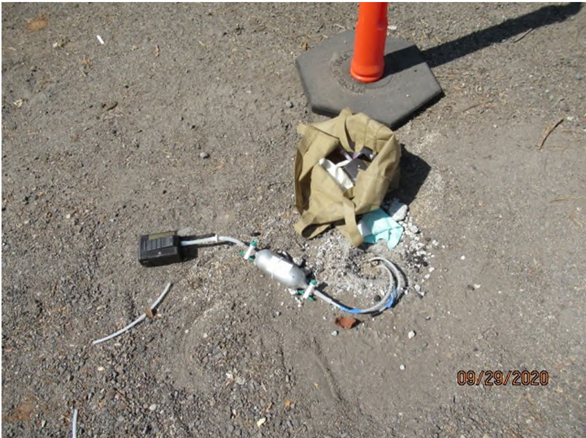
Photo 6 - The collection of the soil vapor sample from the 12-foot probe at SB-7/SVP-7 is shown. The light turquoise colored glove near the probe tubing emerging from the ground has a leak detection compound (isopropanol).
