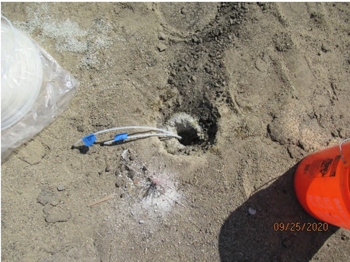
Photo 4 - The soil vapor probes at SB-3/SVP-3 are shown, including 7-foot and 12-foot probes. The shorter tubing at each onsite soil vapor probe location was the 7-foot probe, with the longer tubing the 12-foot probe. The soil vapor probes were labeled with tape as well.
